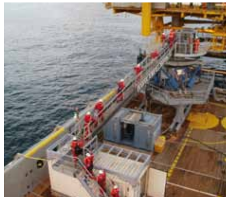
Rig crew "walking to work" using the Ampelmann gangway
